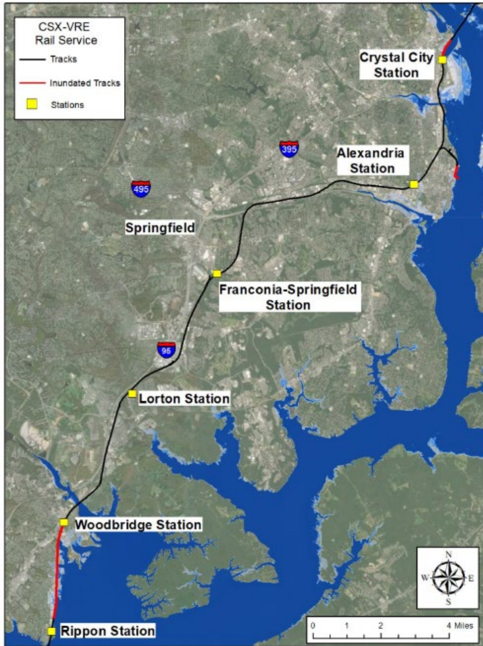
Figure 3-4. CSX Freight and VRE, 1 percent AEP Inundation
