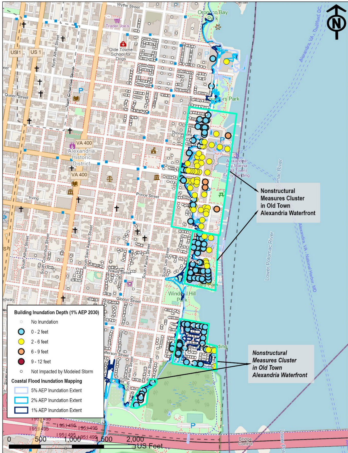
Figure 3-20. Nonstructural Measures Cluster in the Old Town Alexandria Waterfront Neighborhood in the City of Alexandria
