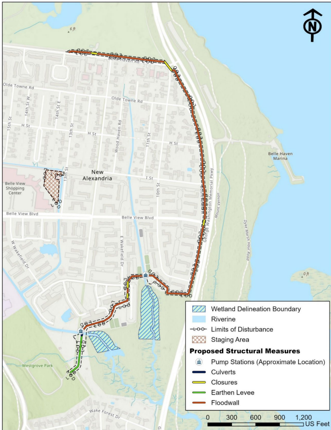
Figure 4-3. Proposed Structural Measures and Limits of Disturbance for Alternative 5c and the Location of Wetlands and Riverine Systems
