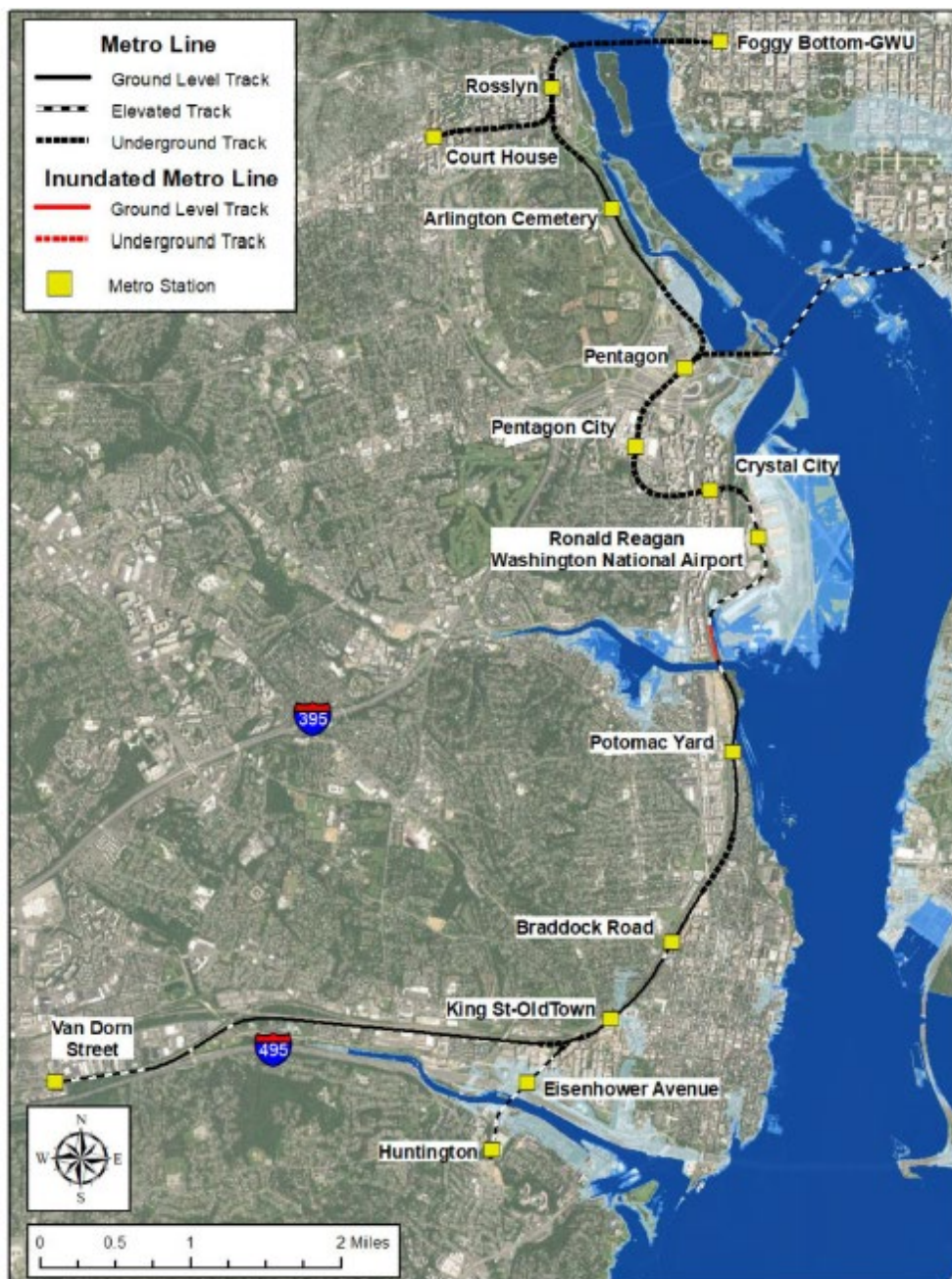
Figure 3-3. Washington Metro Blue and Yellow Lines, 1 percent AEP Inundation Note: Metro railroad track inundation caused by a 1 percent AEP coastal storm under four SLR scenarios.
