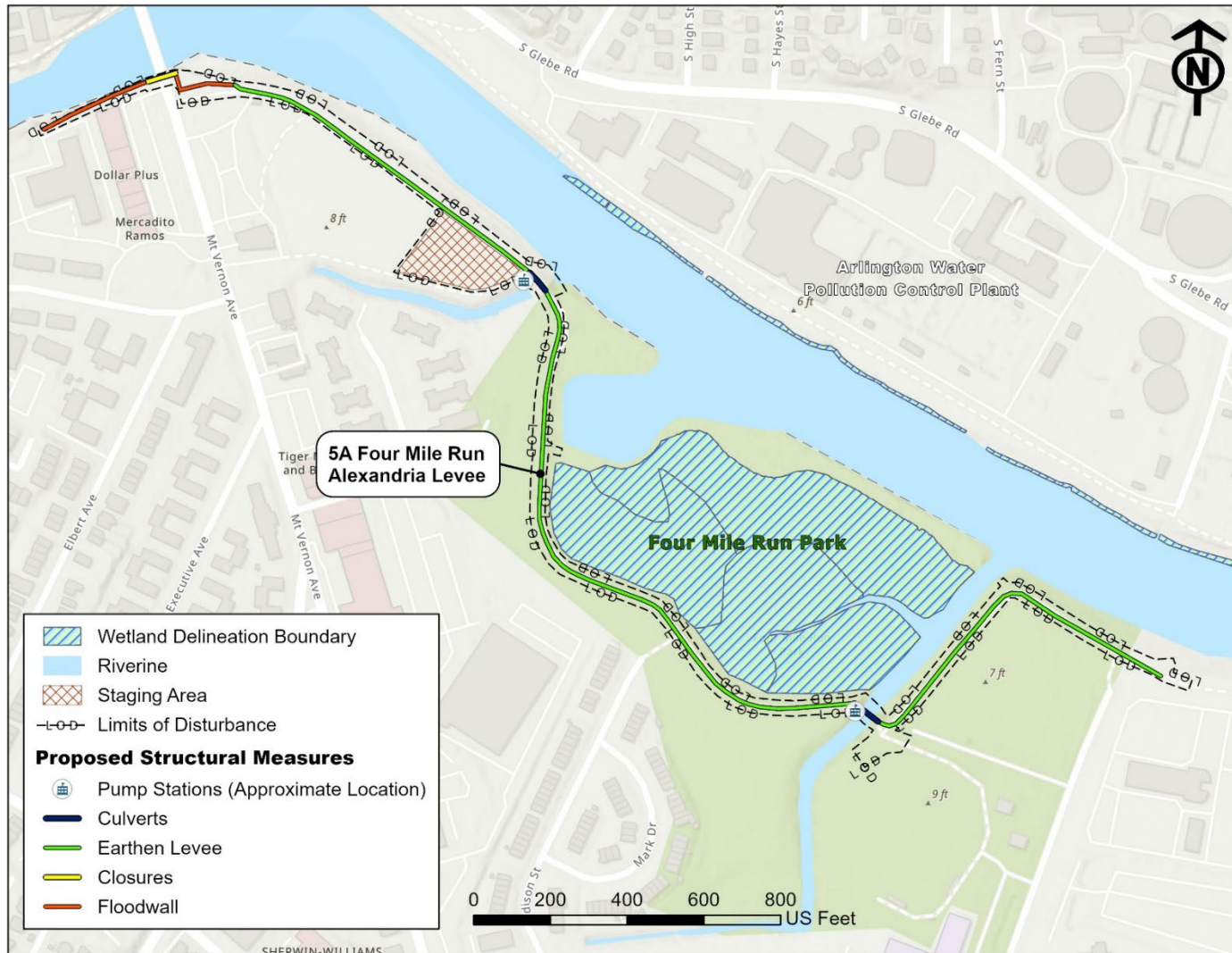
Figure 4-2. Proposed Structural Measures and Limits of Disturbance for Alternative 5a and the Location of Wetlands and Riverine Systems at Four Mile Run
